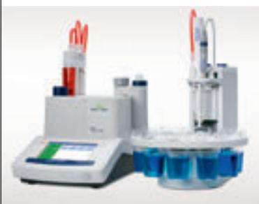
The automatic Rondolino titration stand is simple to install and uses minimal bench space. Series of up to nine samples are processed quickly and safely. Dip-rinsing after each analysis ensures minimal carry-over, and, after the series, the sensor is moved to a fixed conditioning beaker.
