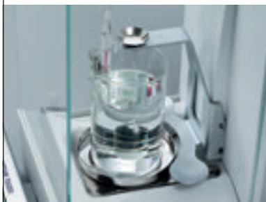
By simply removing the balance weighing pan, the density kit can be installed on your balance in a few simple steps.
