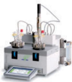
EasyMax makes chemical synthesis easier by eliminating the dependence on ice baths, oil baths, and chillers. Quickly explore reaction conditions, even under low temperatures, while recording data that would otherwise be missed.
