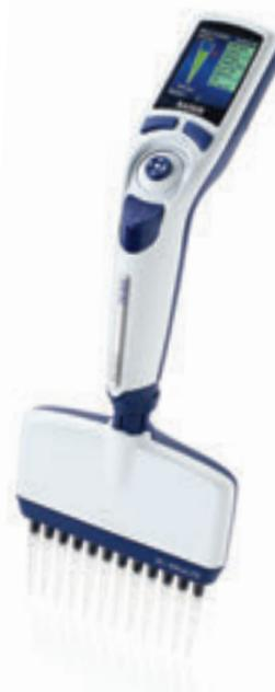
The E4 XLS+ multichannel pipette is a perfect tool for high-throughput work. It is fast loading, lightweight and easy to handle. E4 delivers precision and consistency across all channels. Pipette settings, protocols and service alarms can be password protected for GLP/GMP™ compliance.
