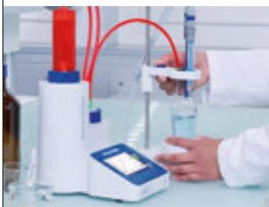
This instrument was specifically designed to simplify sodium determination in food products using the standard addition technique. Simply add a sample and ionic strength-adjustment (ISA) solution and start the measurement. No system calibration is necessary. Specific sodium analysis has never been so quick and easy.
