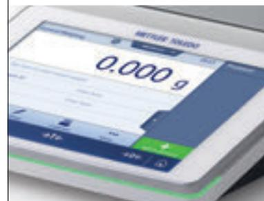
QA functions automatically monitor the balance level, routine tests and the minimum weight limit. The integrated StatusLight™ makes it easy to see at a glance if it is okay to start your weighing task.
