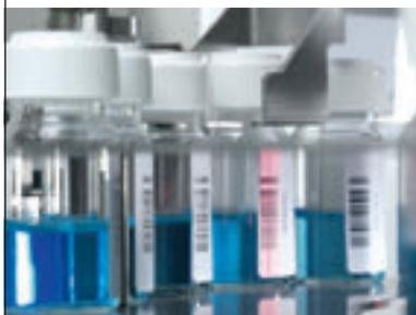
LiquiPhysics™ Excellence is not only able to read barcodes; it can also accurately interpret their information. With Smart Codes containing information about the type of product to be measured, the user simply scans the barcode to start the measurements. There is no additional button to click.
