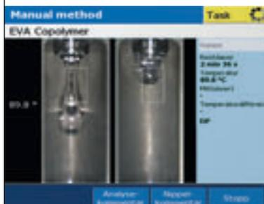
Observe your measurements in real time via video or replay the video to verify your results. Digital image analysis and automatic detection of dropping and softening points guarantee that results are reliable.
