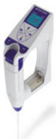
The Densito 30PX and the Refracto 30PX offer all the features required for successful on-site density and refractive index measurements including automatic temperature compensation, direct display of the result in the desired unit, built-in timekeeping for full GLP compliance and data output via infrared interface. Densito and Refracto come with practical carrying cases which contain everything necessary to carry out measurements.
