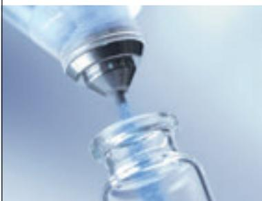
Quantos can dose from one milligram to five grams of free-flowing powder directly into your target container. The highly accurate dosing process eliminates variability and out-of-specification results. Automated dosing can reduce the minimum net sample weight of your balance by up to 30 %.
