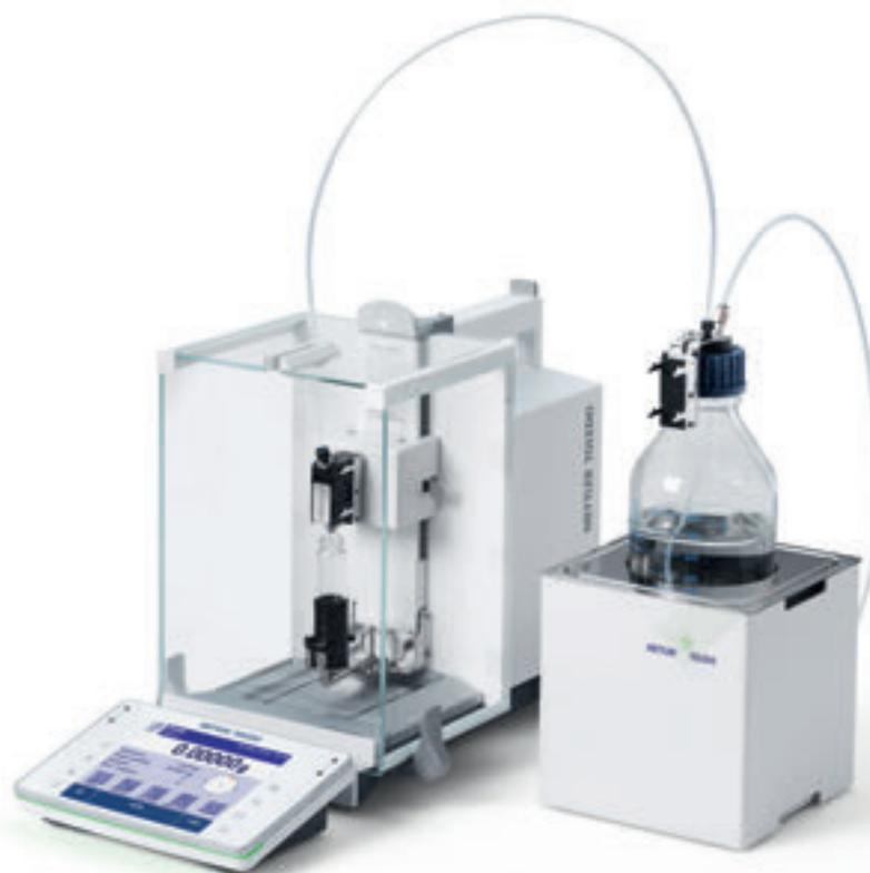
XPE analytical balance with liquid module
