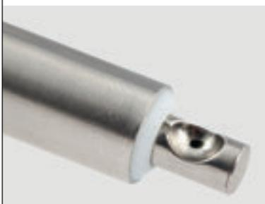
Sampling reactions with precision is challenging, especially for heterogeneous or multiphase reactions. EasySampler samples from the same position in the reactor into a fixed-volume pocket. Solids begin dissolving immediately in the quench step for accurate and reproducible analytical data.
