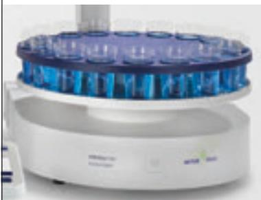
With flexible InMotion™ autosamplers, automated sensor calibration and measurements of up to 303 samples are possible. Professional automation ensures security, comfort and maximum efficiency.
