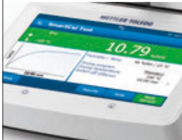
Simply select the integrated SmartCal method on the instrument, distribute the contents of the test sachet evenly over the sample pan and start the measurement. After ten minutes, you know if your instrument's performance is satisfactory or not.
