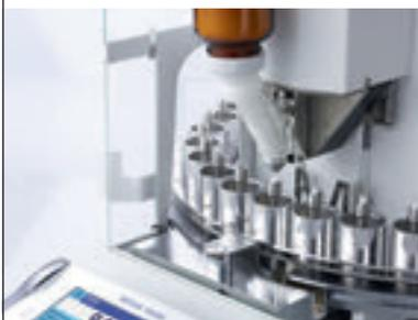
Automated powder dosing is much faster than dosing manually, capturing huge time savings for your lab. Up to 30 samples can be dispensed in one completely unattended run. While the autosampler is at work, your staff can focus on other tasks.
