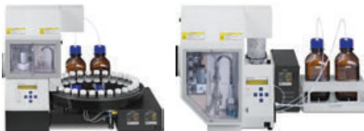
SC automation units are available in heated versions suitable for performing density measurements of samples which are highly viscous or even solid at ambient temperature such as paraffins, bitumen, heavy crude oils and edible fats. The SC1H and the SC30H can handle samples with a melting point of up to 60 °C.
