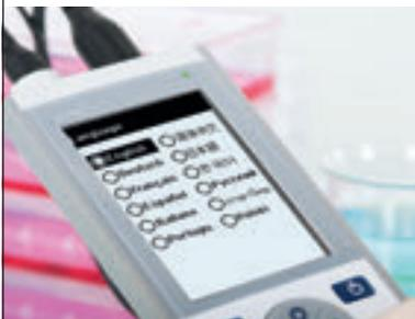
Seven2Go's new intuitive menu guarantees out-of-the-box operation for anyone. Thanks to ISM, the sensor is automatically recognized to save time and reduce errors when changing the sensor.
