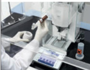
Potent or toxic compounds remain sealed within the dosing head and hence aerosol formation is kept to a minimum. With an automated dosing process, users work safely without exposure to substances during weighing.
