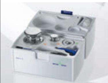
The larger test weight (1) at approx. 100 % capacity assesses systematic deviations (sensitivity offset). The smaller test weight (a) at approx. 5 % capacity assesses random errors (repeatability, shown in red). Low test loads (b) are not recommended.
