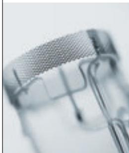
For most samples, a generator without a diaphragm is easy and convenient. No catholyte is needed and the anolyte can be exchanged with the solvent manager in One Click™.
