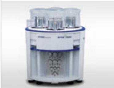
The absolute highest accuracy can be achieved by utilizing automated mass comparators. As air density is one of the primary contributors to uncertainty, the portfolio covers vacuum, constant-pressure and ambient-pressure models.
