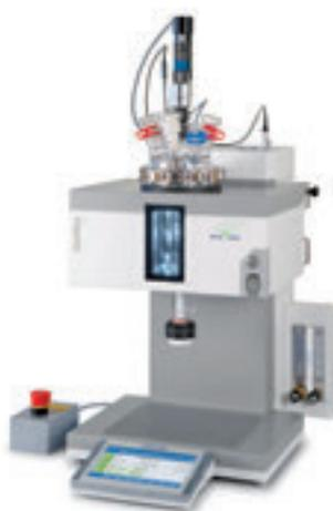
OptiMax ensures robust and scalable processes by applying synthesis reactors on the liter scale. Unattended control increases productivity while ensuring that all data is collected and experiments are safe. A HFCal option ensures scale-up issues are identified earlier.
