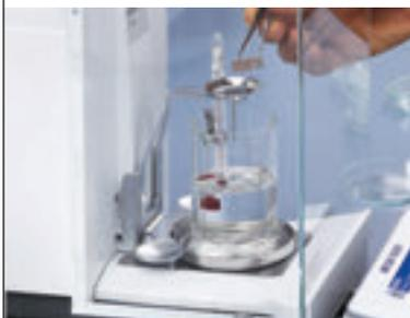
The built-in application on XPE and XS balances provides user guidance, collects results, calculates density values and allows statistical evaluation of a measurement series. Five methods are included.
