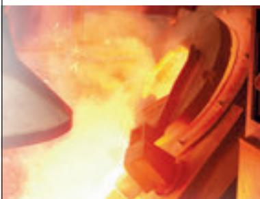
Our specially produced super-austenitic stainless steel is cast under vacuum to reduce undesired trace elements, remove dissolved gases and improve oxide cleanliness. This optimizes the physical properties of the steel; e.g. density is highly reproducible.
