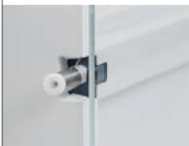
The compact AntiStatic Kit for XPE analytical balances is easily configured to activate when the draft shield doors are opened.
