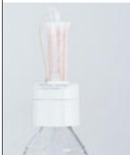
The solvent manager takes care of filling, draining and exchange of reagents. It is controlled by the titrator and full security is guaranteed by the overflow protector in the waste bottle.
