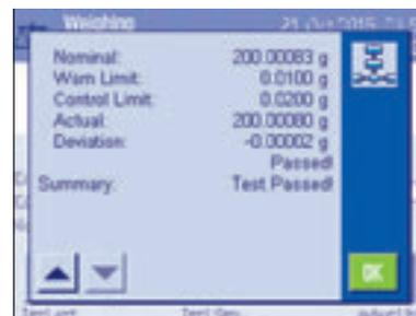
Routine balance-testing maintains balance accuracy to limit the risk of working outside your specified process tolerances. CarePac weights are specified to validate process tolerances up to 0.03 %.
