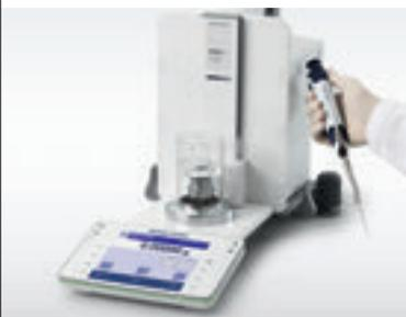
With an RFID-tagged pipette, the check is automatically initiated. The tag contains the pipette data, check interval and method. When a check is passed, the next date is stored on the pipette.
