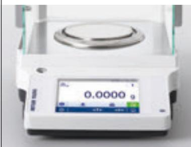
The large 4.5-inch color TFT touchscreen with clear icons and intuitive guidance enables users to operate the balance efficiently even while wearing cloth or rubber gloves. Multilingual text and graphics walk you through every step of your weighing procedures.
