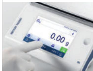
The large 4.5-inch color TFT touchscreen with clear icons and intuitive guidance enables users to operate the balance quickly even while wearing cloth or rubber gloves. Multilingual text and graphics are included.
