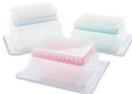
Green-Pak refills are completely sealed, eliminating contamination. The filter and sterilized tips are irradiated and certified free of DNase, RNase, DNA, endotoxin, ATP, PCR inhibitors, protein and protease. These refills also offer fast, trouble-free loading. Available standard, sterilized or sterilized with aerosol-resistant filter tips.
