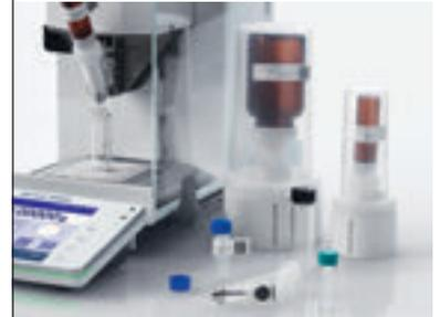
A transport/storage box protects your dosing heads when not in use and ensures that valuable and toxic substances remain safe. The transport container is impact-resistant and water-tight for safe storage.
