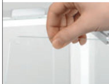
The QuickLock draft shield dismantles in seconds without any tools and all parts are dishwasher-safe. Surfaces are smooth and rounded to make cleaning easy.
