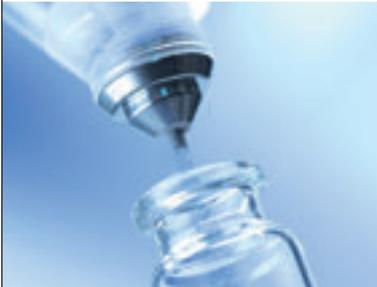
A highly precise mechanism guarantees homogeneous powder flow. The dosing head learns powder behavior and optimizes dosing accuracy and speed. While no configuration is needed, any target weight can be hit.
