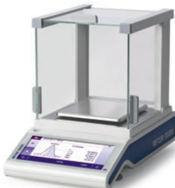
MS603TS 1 mg precision balance with draft shield
