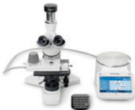
Microscope equipped with Hot-Stage 84
