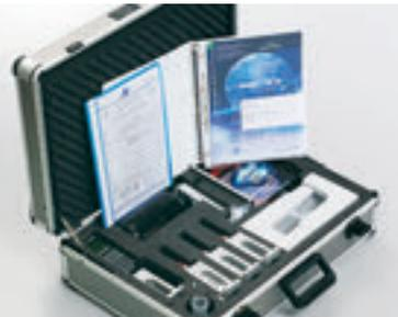
Calibration is essential for getting accurate and reliable titration results. Traceable calibration tools ensure that the titrator functions according to its operational specifications. A calibration certificate provides the required evidence for quality audits.
