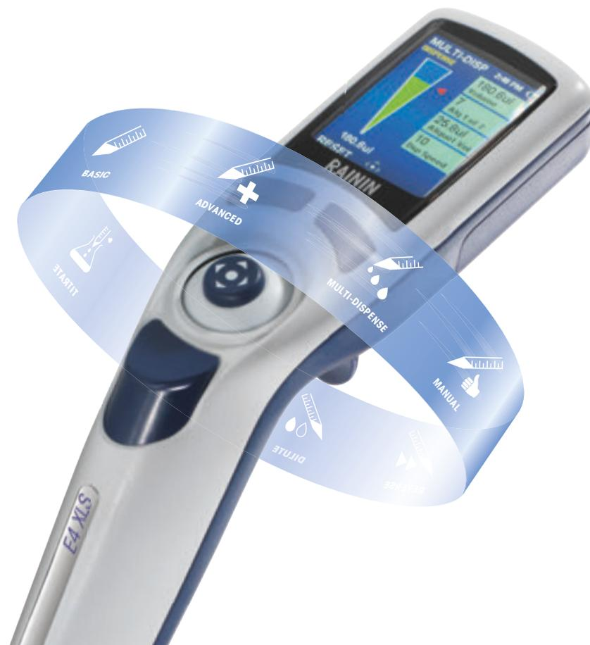
The E4's carousel-like menu makes switching between features and functions fast and easy.
