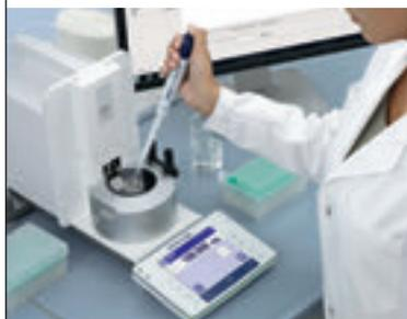
The Calibry-Software cockpit screen ensures efficient pipette calibration workflows in accordance with ISO 8655. User management, audit trail and a secure database help ensure compliance with FDA 21 CFR Part 11.
