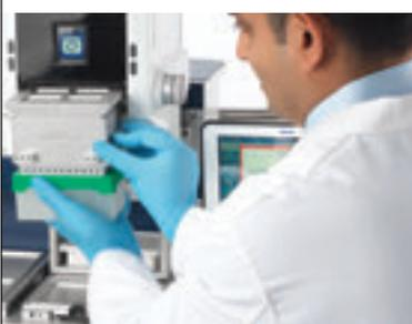
Quickly replaceable liquid heads provide great flexibility. Get the precision you demand with the 0.5–20  $\mu\text{L}$  head, the daily workhorse you need with the 5–200  $\mu\text{L}$  head and the multi-dispensing capability of the 100–1,000  $\mu\text{L}$  head.
