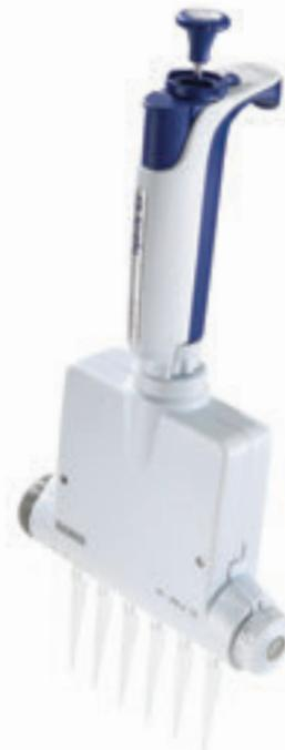
Pipet-Lite XLS Adjustable Spacer pipettes let you set nozzle spacing for use with 24-, 48- or 96-well plates with just a twist: 9–19 mm on 6-channel and 9–14 mm on 8-channel models. The liquid end rotates 360° for quick alignment with the plate.
