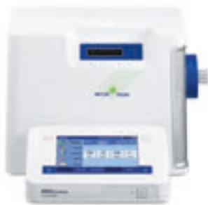
DM density meters determine the density and/or specific gravity of liquids quickly and accurately. The results are automatically converted into one or several pre- or user-defined units such as Brix, API degrees or alcohol concentrations. Automatic error detection, entire temperature range adjustments and built-in algorithms shorten measurement times required by up to 75 % – DM and DX are doubtlessly the state-of-the-art pinnacle for digital density measurement.
