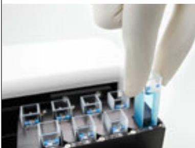
This auto-changer offers you efficient automatic measurement of series of up to eight cuvettes for both standard measurements with blank subtraction or complex kinetic applications, thermostatable from 10 °C to 80 °C.
