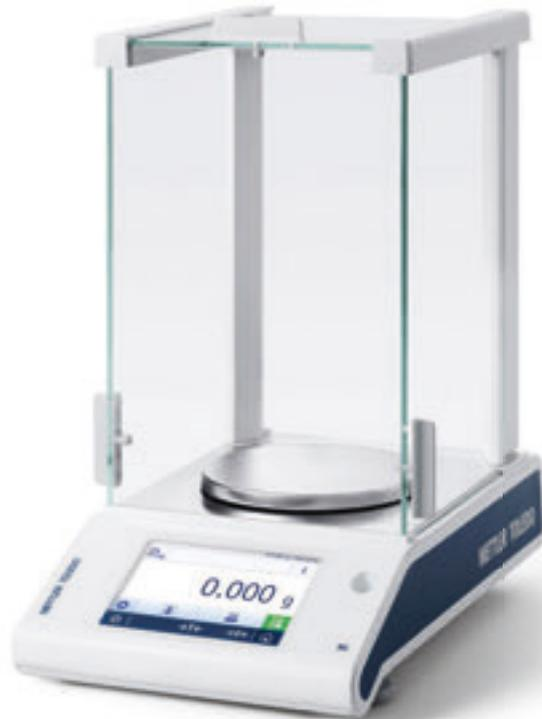
ML503T 1 mg precision balance with draft shield
