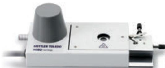
**Hot-Stage microscopy is a powerful tool that is widely used for the visual characterization of all kinds of thermal transitions. The possibility of directly observing morphological changes in a sample as it is heated or cooled is of enormous value. Changes in the shape, structure and color of crystals are seen as well as their size and number. The technique allows phase transitions to be characterized and provides information on expansion and shrinkage behavior.**
