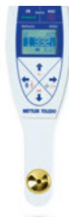
The Refracto 30GS features a very wide measuring range and a quick temperature response thanks to its special measuring cell equipped with a gold-plated stage ring and a prism made of artificial sapphire. This allows even faster measurements in any environment.
