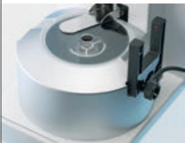
The light barrier enables the evaporation trap lid to open automatically, reducing handling steps and providing fast, stable results. In combination with the 100 mL tank, many calibrations can be carried out in a continuous process.
