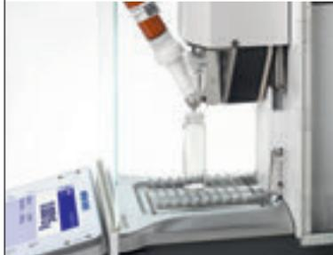
Powders are sealed within the dosing head. Individual dosing heads for each powder eliminate the risk of cross-contamination. Once the dosing head is filled, work proceeds with no powder contact.
