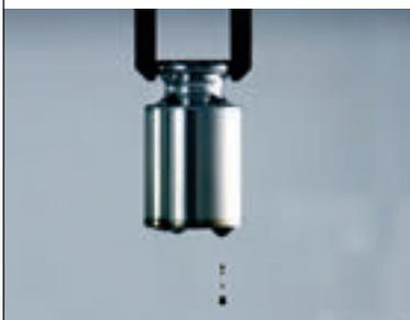
A proprietary process eliminates microscopic protrusions in the weight's surface which is far more even compared to mechanical polishing. Thanks to the enhanced properties of the passive oxide film, long-term stability of the weight is improved.
