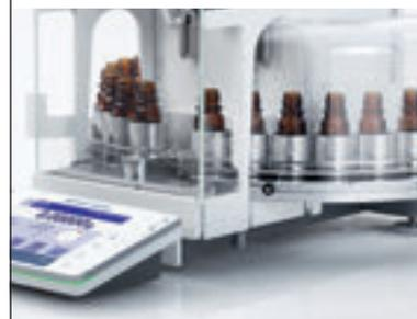
Preparing samples with the Quantos autosampler module is not only considerably faster than preparing samples manually, but it also reduces errors and variability. Different sized containers as well as capsules and vials of any kind are filled quickly and automatically.
