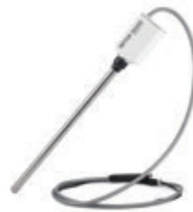
This real-time, probe-based microscope provides instant critical insight into crystal, particle and droplet systems. It enables chemists and engineers to detect and understand process changes that could take months to discover with traditional offline microscopy techniques.
