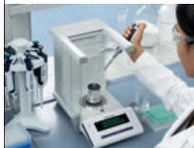
Quickly convert your semi-micro balance into a pipette checking station by installing an evaporation trap. The built-in application guides you through the pipette check process.
