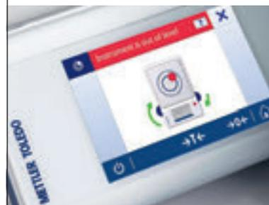
The built-in LevelControl function issues a warning when the balance is not level and provides onscreen guidance to help you level the balance in seconds.
