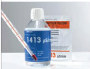
Depending on the type of sensor, conductivity standards are used for calibration or verification. Low-conductivity standards have a limited lifespan and require special handling. They are intended for verification purposes. Our sachets guarantee fresh solution for every calibration as well as maximum ease-of-use.
