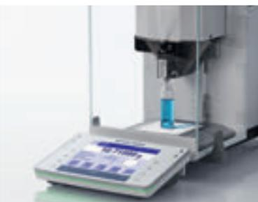
This gravimetric sample preparation uses precise balance results to produce accurate concentrations, in contrast to error-prone visual readings when using volumetric flasks. Automatic results recording also eliminates transcription errors.
