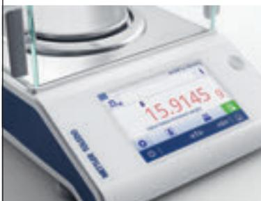
The weight value remains red until the net sample weight is above the pre-programmed minimum value. A user-defined minimum weight can also be programmed into the balance to provide an additional safety factor.
