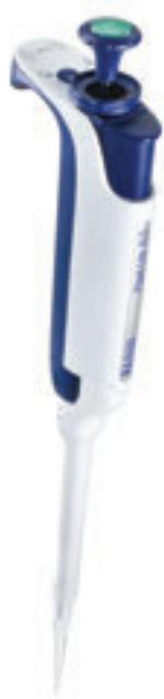
Pipet-Lite XLS+ further reduces plunger force and tip-ejection forces. Eleven models cover volume ranges from 0.1  $\mu\text{L}$  to 20 mL; custom fixed volumes are also available in LTS and traditional models. The RFID tag in every XLS+ model makes calibration and pipette inventory-management easy when used with SmartStand.
