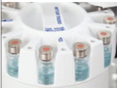
After quenching, the liquid handling system dilutes the sample to a user specified concentration and transfers it to a vial, ready for offline analysis. Quench and dilution steps can function as sample derivatization steps, thus decreasing sample preparation time and eliminating human error.
