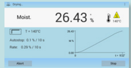
Real-time graph of ongoing drying process
